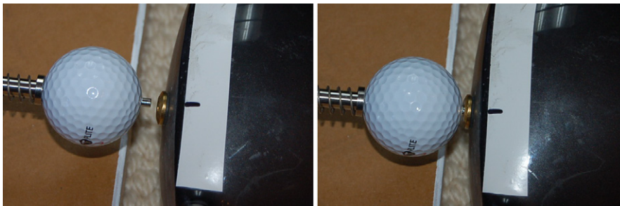
Picture 4. Small plate with a hole (diameter five mm) is adhesively attached to the sweet spot and is then, while practicing, precisely aligned to the pin (four mm).
